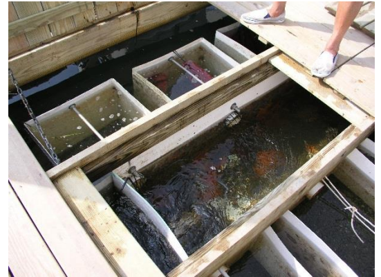
Figure 2 A FLUPSY or Floating Upweller System
