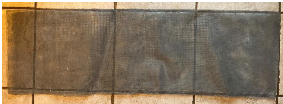
Figure 5 Window screen stitched nursery bag with two separate sides created by a stitched divider in the center
