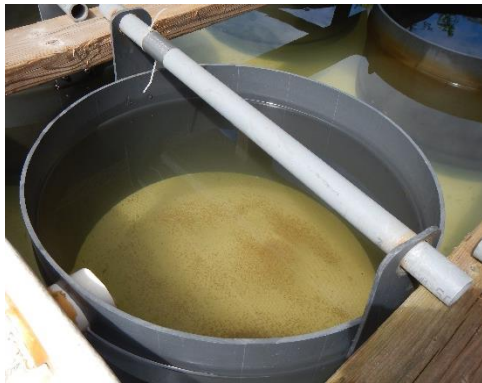
Figure 4 Upweller silo from a land based system
