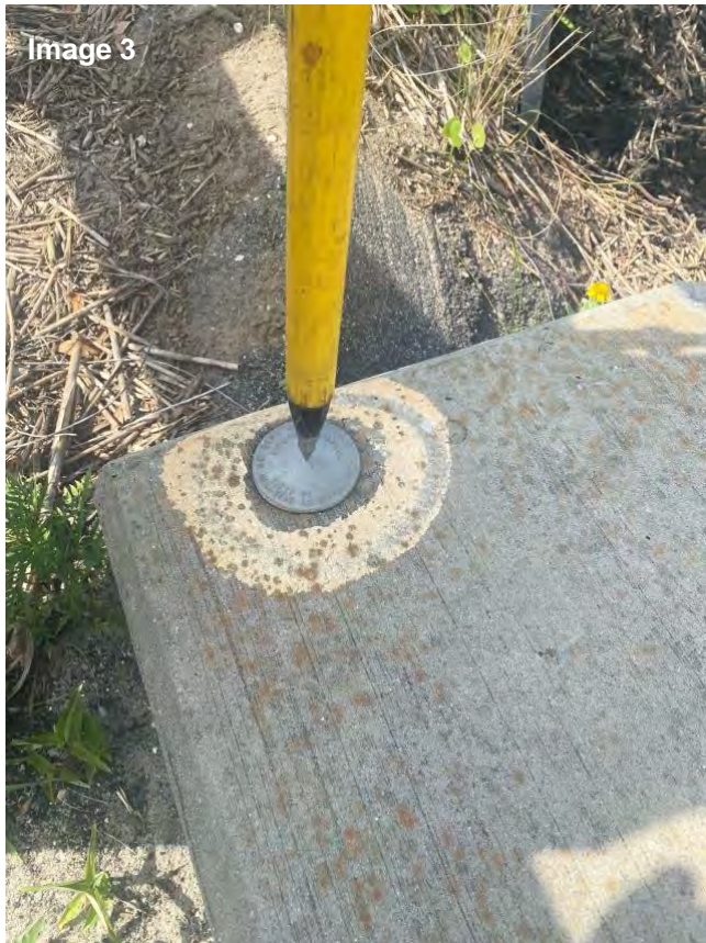
Image 3: North Carolina DOT benchmark with RTN placed vertically above the BM. Note the DOT metal disc has yellow paint around it to help identify it more easily.
