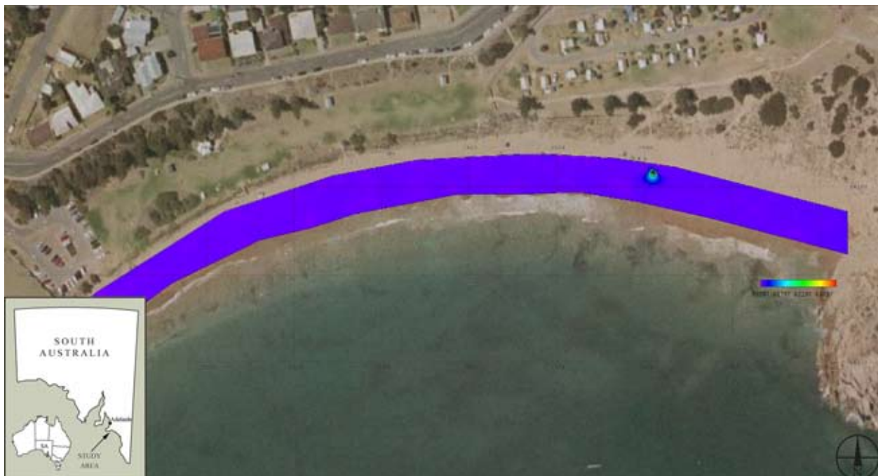
Figure 2. Horseshoe Bay reconnaissance magnetometer map overlaid on an aerial photograph. Grid lines are easting and northing with a spacing interval of 50 m. (Map by authors).
