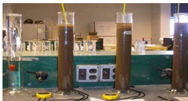
Figure 4. Hydrometer set up (Photo by Maik Pertermann, 2005).
