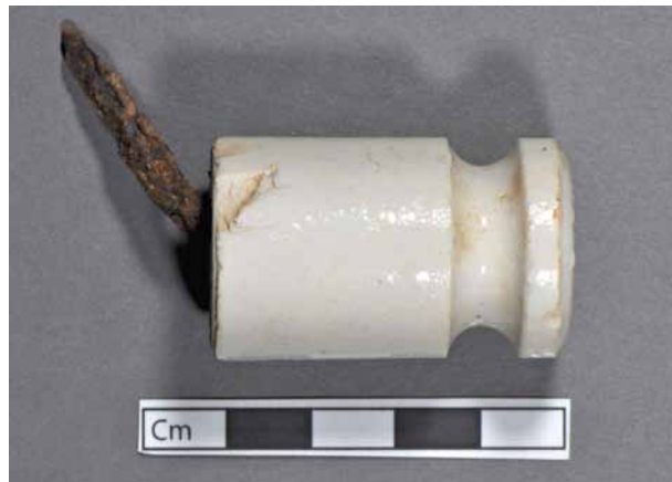
Figure 4. Nail knob with nail still present, excavated at Stanford University, courtesy of Laura Jones. (Photo by author, 2010.)
