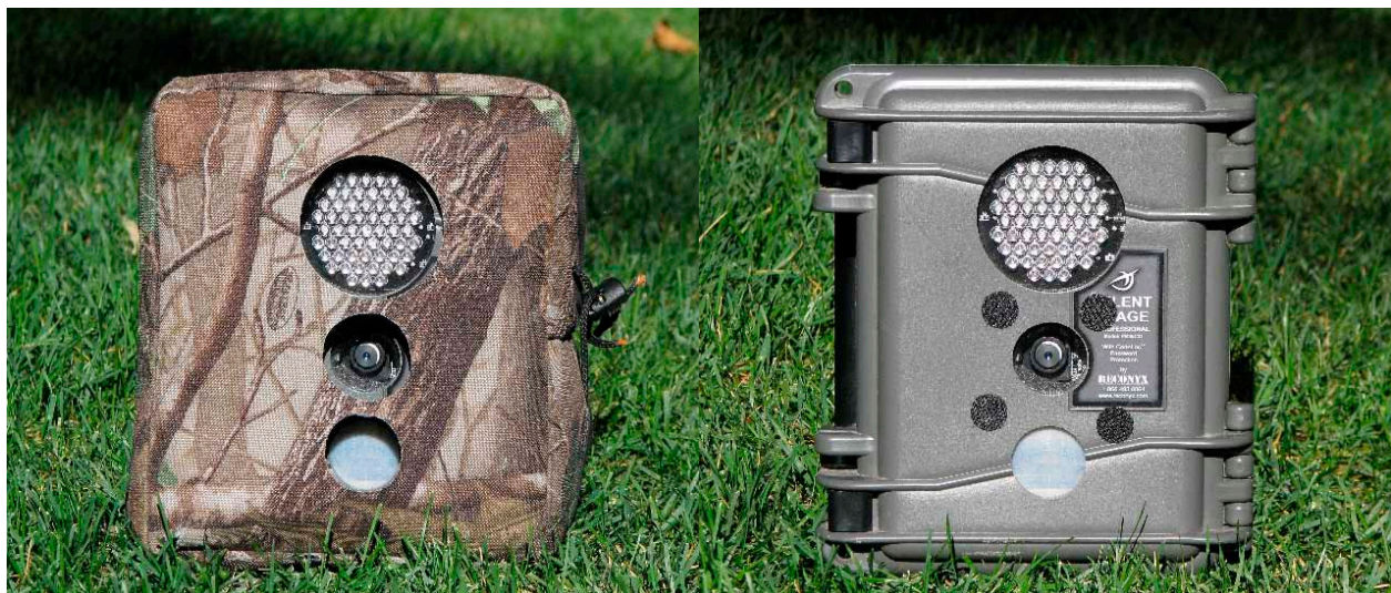
Figure 2. Reconyx PM35C31 Silent Image Professional camera measuring 8.75 in. high, 7.5 in. wide, and 4 in. thick, with (left) and without camouflage (right). (Photo by Don Merritt, 2010.)
