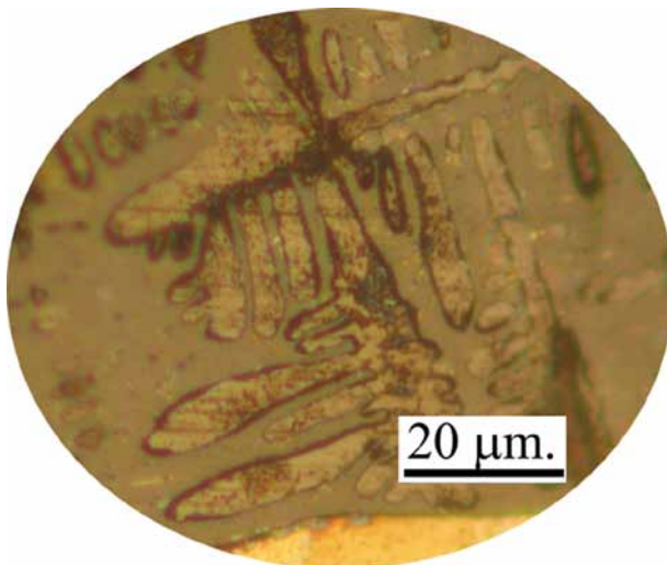
Figure 10. Enlarged detail of Figure 8, showing ferritic structure and nonmetallic inclusions in Area B. (Photo by Maria Lucchetta, 2010.)
