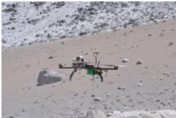
Researchers perform a test flight of a MultiGAS-equipped Matrix Quadcopter. The instrument, which measures atmospheric carbon, was used by DCO scholars on their "Trail By Fire" expedition, a 4,000-kilometer voyage from Peru to Chile that aimed to help quantify and model volcanic carbon emissions.
