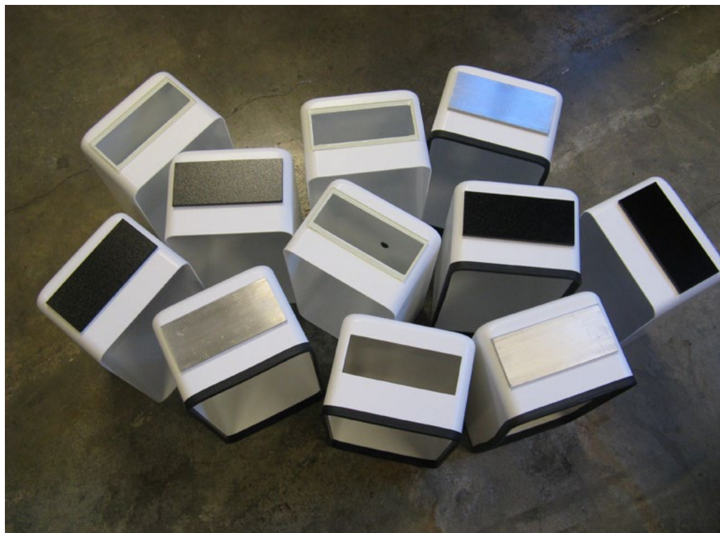
Researchers at the University of Oregon's Center for Biology of the Built Environment used these airtight microcosms to study how different wavelengths of light affect microbial community composition in dust. (PHOTO COURTESY OF THE UNIVERSITY OF OREGON)
