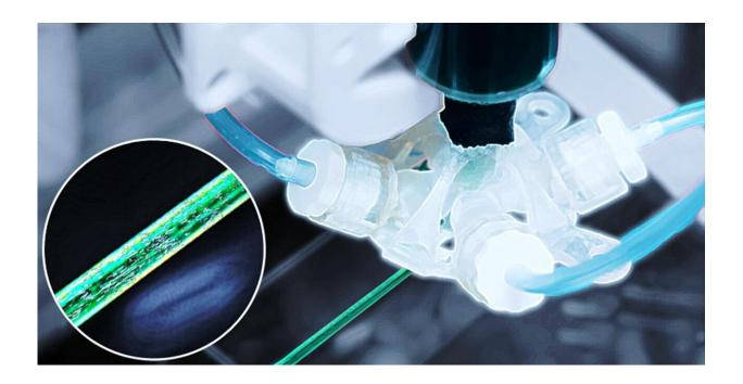
The morphing nozzle in action, 3-D printing fiber-filled composite materials with on-demand control of fiber alignment for "4D printing. Credit: University of Maryland
