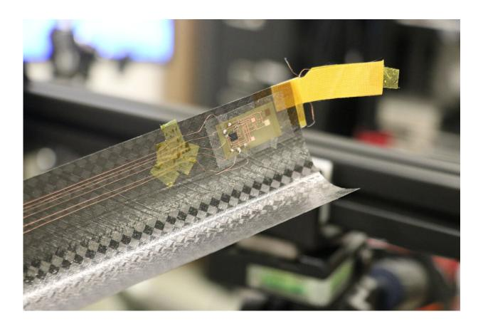
A close-up of the extended boom showing a lightweight, flexible electronics patch with a motion sensor, and a temperature sensor mounted on the boom tip. Credit: University of Illinois at Urbana-Champaign
