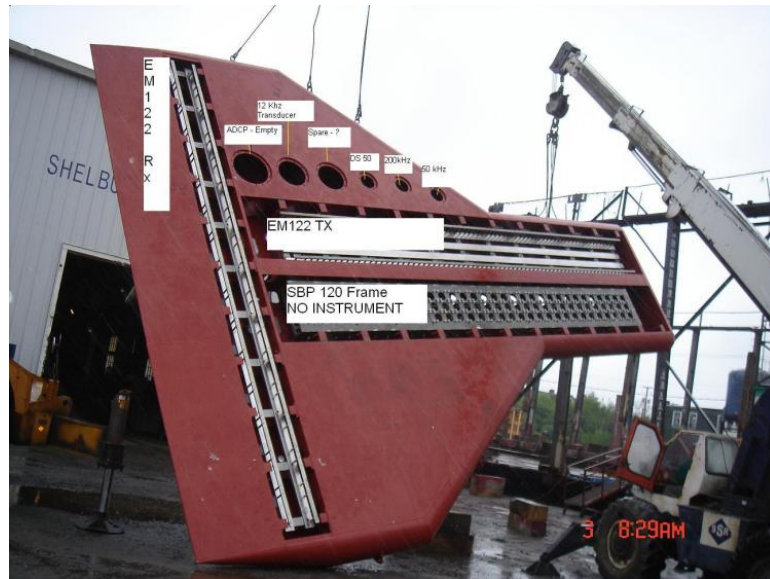
Figure 2.2: Gondola containing a 7 m long array of transducers (EM122 TX) that are oriented parallel to the keel of the ship and a 7 m long array of hydrophones (EM122 RX) perpendicular to the keel. This system is a Kongsberg EM122 multi-beam sonar being mounted on the hull of the RV Langseth. (Photo credit, John Greene, [ Seeing with Sound ]).
