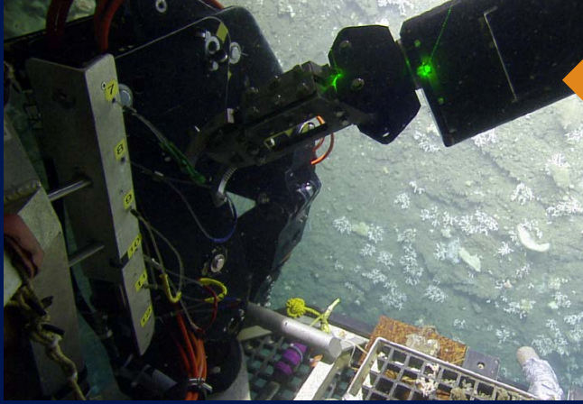
Figure 3. ROV Hercules captures a water sample for eDNA analysis in an onboard Niskin bottle along a canyon wall covered in Lophelia coral.
