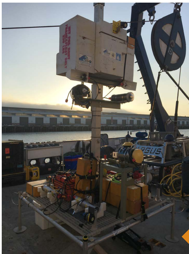
Figure 1. The Autonomous Biogeochemical Instrument for In Situ Studies (ABISS) prototype shown here is equipped with a suite of cameras as well as an optical modem for transmitting HD video and still frames in real time to ROV Hercules .
