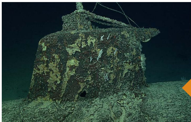
Figure 1. The Japanese mini submarine sank when USS Ward fired a four-inch shell that smashed through the conning tower (hole at base), sinking the mini submarine and two-person crew before its deadly mission could be carried out.
