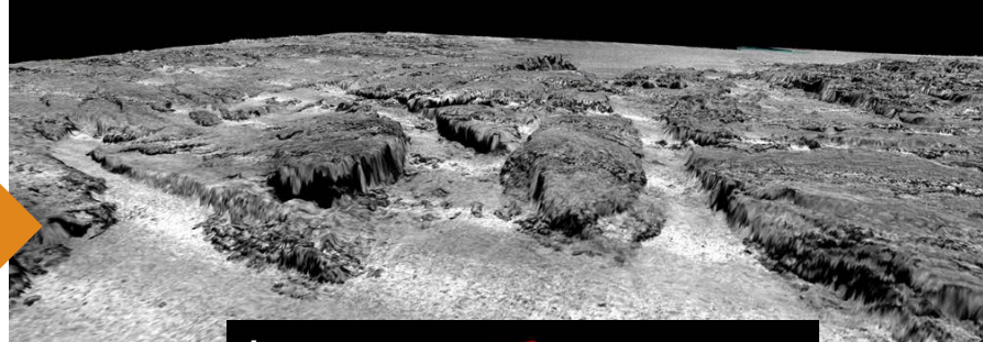
Figure 4. (a) (top) Bathymetry (8–80 m depth, 25 cm grid, 1.5x vertical exaggeration) and (bottom) backscatter (50 cm grid, 1.5x vertical exaggeration) draped over bathymetry data from the ASV provided targets for divers to investigate. (b) The feature identified by the red flag is a cave (40 cm grid, 1x vertical exaggeration).
