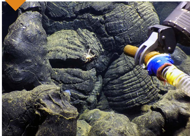
ROV Hercules prepares to take a suction sample of a galatheid crab on a pillow basalt outcrop on the slope of Socorro Island, Revillagigedo Archipelago, Mexico, from E/V Nautilus cruise NA092. Image credit: D. Fornari (WHOI-MISO Facility) and OET
