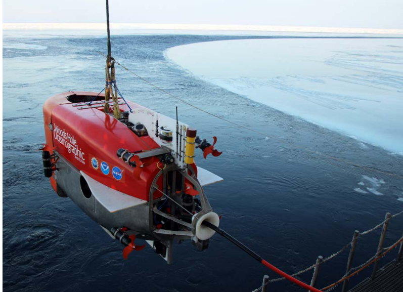
FIGURE 1. The WHOI-developed Nereid Under Ice (NUI) hybrid autonomous vehicle is ready to dive into the Arctic Ocean during the Hot Vents in an Ice-Covered Ocean (HACON) expedition. Image credit: Stefan Buenz, Norges Artiske Universitet
