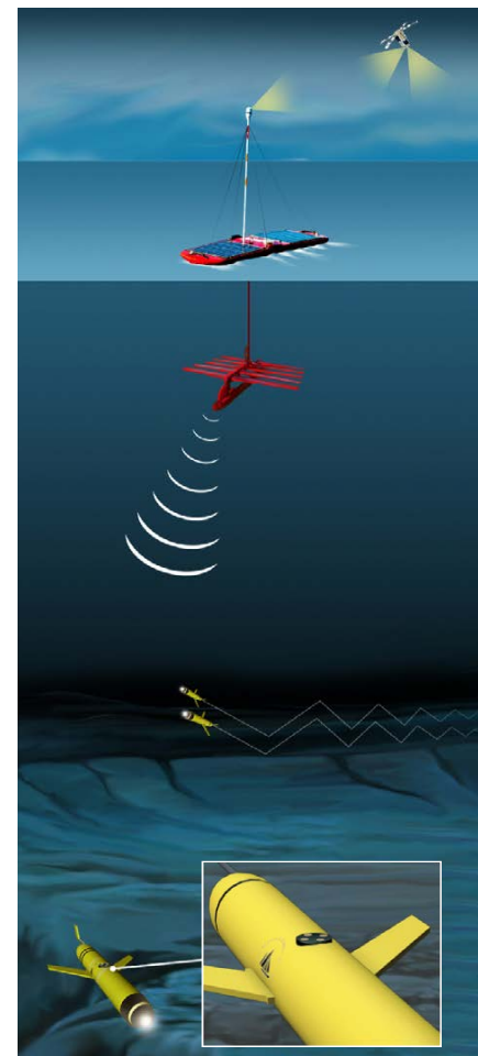
FIGURE 4. Illustration of a glider equipped with a one-way-travel-time inverted ultra-short-baseline transducer that "listens" for a signal from the surface to determine the glider's location. Image credit: WHOI
