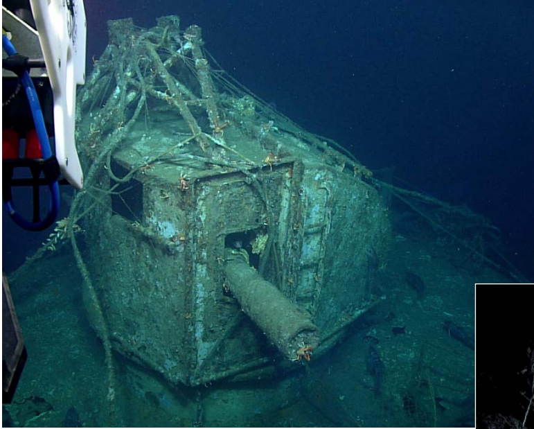
FIGURE 3. ROV Deep Discoverer locates USS Baldwin 's gun fire-control system by targeting the antenna array and cylindrical range finder located above the pilot house. Note the derelict fishing gear on the wreck. INSET. High-resolution 3D point cloud rendering from the SeaVision laser imaging system. Image credit: Kraken Robotics and NOAA OER
