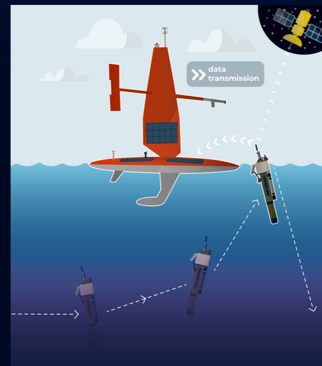
FIGURE B5. During a rendezvous between a saildrone and a surfacing BGC-Argo float, the USV would record data from the float and simultaneously make p\text{CO}_2 measurements. Data files too large to be transmitted to satellites by the float (e.g., particle and plankton images) could be transferred to the USV for later downloading when it returns to port. Licensed under CC BY-SA 4.0 by Thomas Boniface
