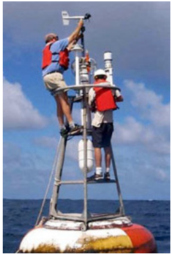
Remote Automated Weather Stations transmitting to GOES
