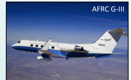
Non-pressurized pod with air inlets for cooling the radar electronics
