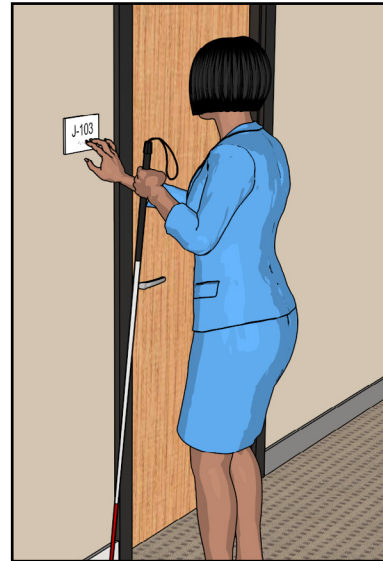
Braille is located below raised characters, including when text is multi-lined.
