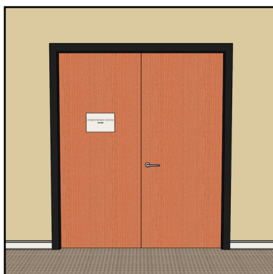
Sign on inactive leaf at double-door entry
