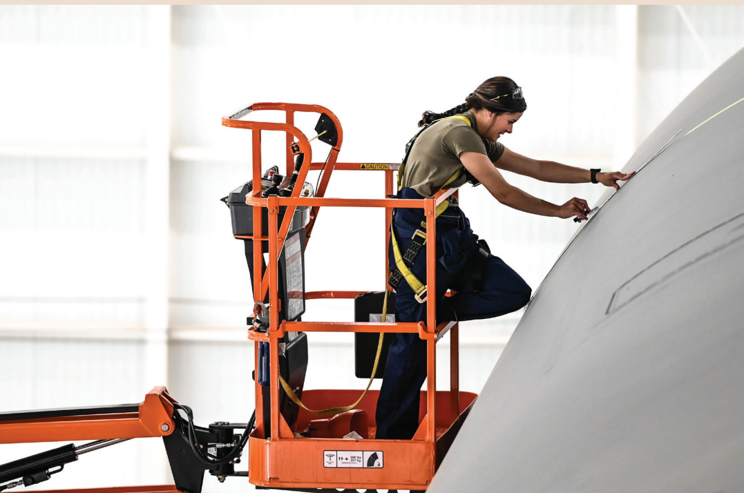
Tech. Sgt. Michelle Rozich, 911th Airlift Wing aircraft structural technician, tapes off the fuselage of a C-17 Globemaster III before painting on WWII invasion stripes, June 6, 2023, at Pittsburgh International Airport Air Reserve Station. When it finally came time to paint, Airmen broke into teams and used screen ink thinned with acetone to apply the stripes. (U.S. Air Force photo by Master Sgt. Jeffrey Grossi)
