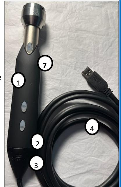
To attach a lens, match up the attachment to the holes on the top of the camera and turn to the right to lock into place
