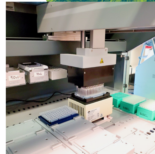
TOP A choanoflagellate is a microscopic organism that Bigelow Laboratory scientists have shown can consume viruses directly as food. BOTTOM Robotic equipment processes samples at the Single Cell Genomics Center, which sorts and analyzes the genetic information of individual cells and viruses.
