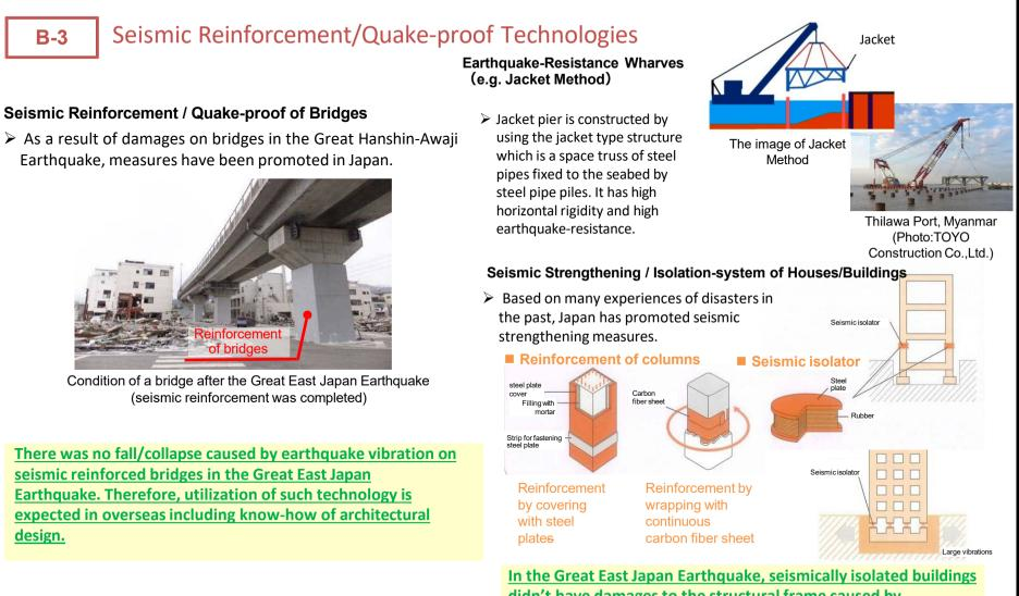
didn't have damages to the structural frame caused by earthquake motion, and proved the effectiveness to the major earthquake.
