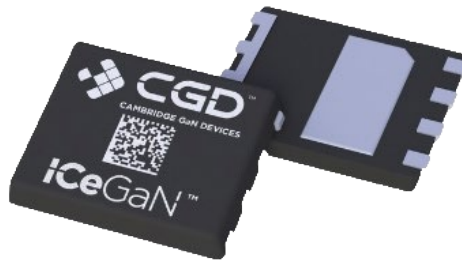
CGD's GaN-on-silicon power transistors
