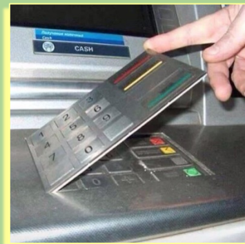
Photo 19: External Skimmer - Keypad Overlay
