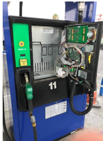
Photo 24 and 25: Fraudulent Card Reader and Internal Skimmer Detected and Removed from Inside a Gasoline Dispenser Cabinet
