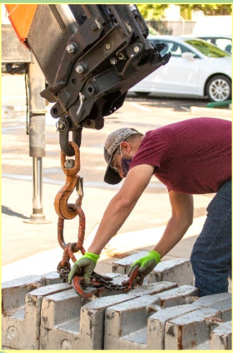
Photo 15: 500-pound Standard Weights Being Offloaded by a Crane Truck to be Certified at DMS
