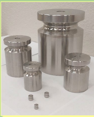
Photo 14: Variety of Standard Weights Ranging from 1 gram to 5 kilograms
