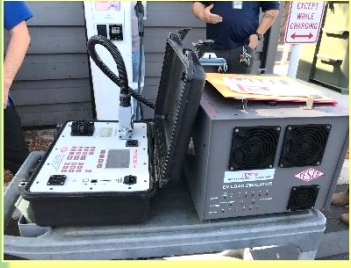
Photo 33: DMS' EVSE Field Test Standard Used During a Training Course in San Joaquin County
