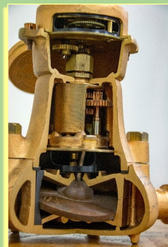
Photo 17: Cross-Section Cutaway of a Commercial Water Submeter Used for Training Purposes
