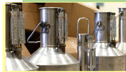
Photo 16: 5-gallon Standard Measures to Test the Delivery of Liquid Fuel (Prover)
