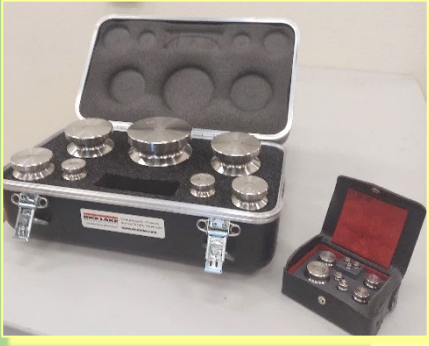
Photo 13: Class F Standard Weight Kit for Testing Commercial Scales
