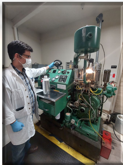
Photo 12: DMS Staff Testing Gasoline Samples to Calculate Octane Rating
