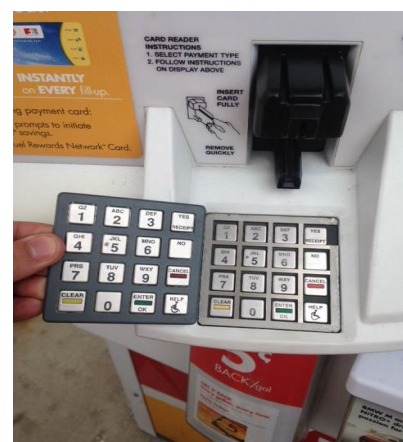
Photo 10: Skimmer – External, keypad overlay
