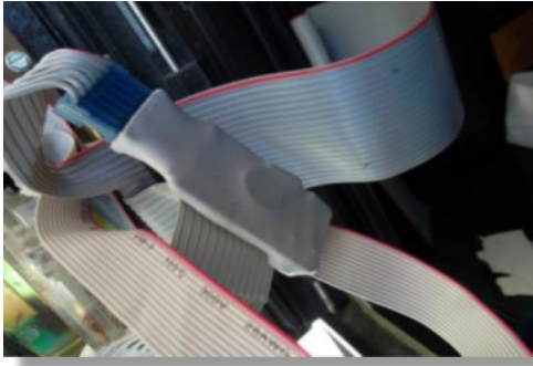
Photo 11: Skimmer – Internal, wireless communication
