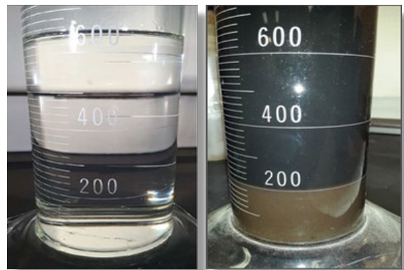
Photos 13 and 14: Compliant gasoline on left. Adulterated gasoline on right
