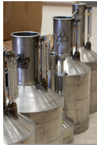
Photo 2: 5-gallon standard measures to test the delivery of liquid fuel (prover)
