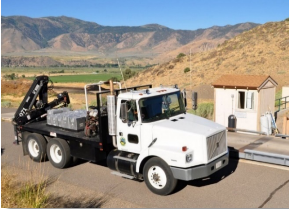
Photo 4: Testing a vehicle scale using certified standard weights Source: N. Reade, Inyo/Mono County Sealer
