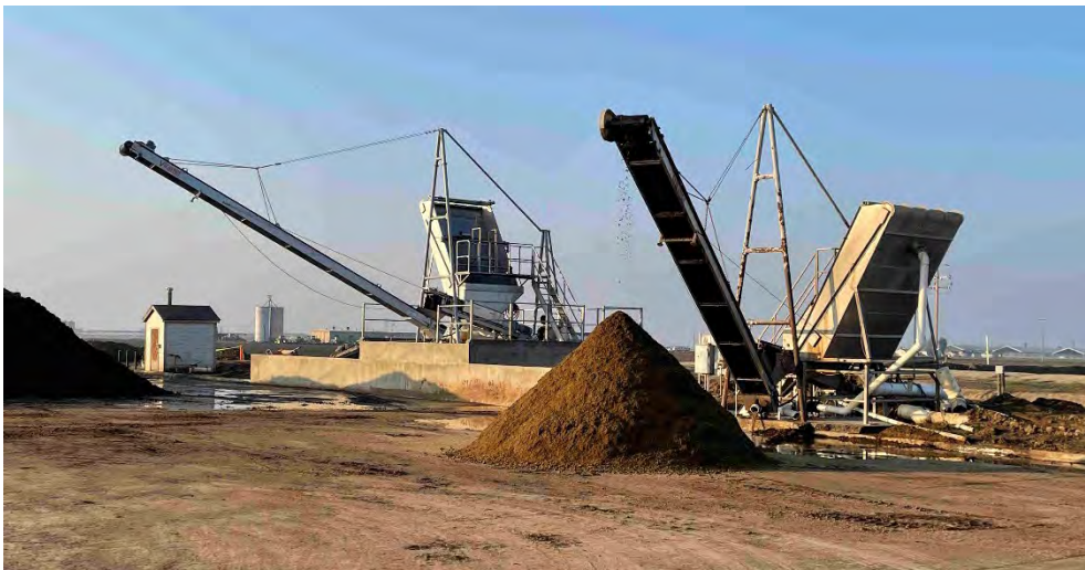
Image 68. Mechanical solid separators at Rib-Arrow Dairy.
