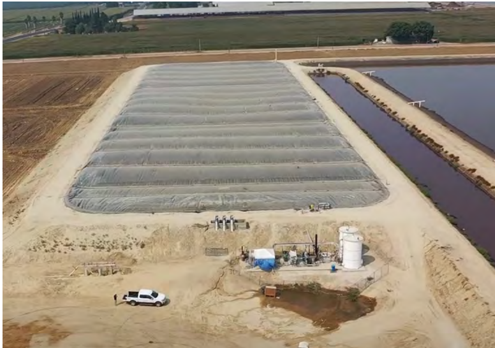
Image 23. Aerial view of the covered lagoon digester and the biogas conditioning equipment at Double D Dairy.
