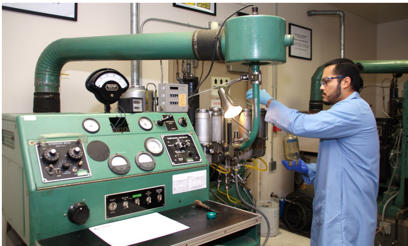
Octane Engine: An Official Test Engine Used to Determine Octane Rating of Gasoline
