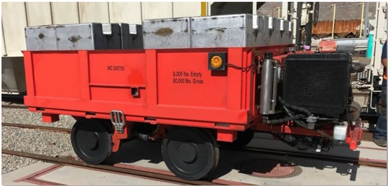
80,000 lb Test Unit Used for Certifying Railroad Scales
