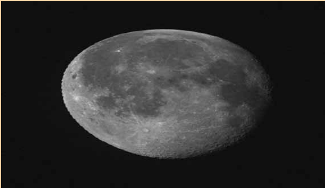
Figure 4: An example of an image of the moon captured from GOES-15. The elongated nature of the image is due to the un-equal horizontal and vertical sampling of the GOES Imager.
