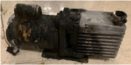
Image of the vacuum pump after the explosion from the University of Pennsylvania's EHR website
