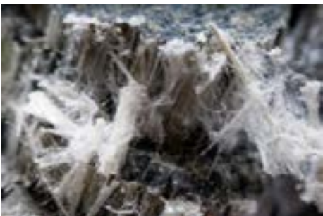
Asbestos chrysotile fibers as seen under a microscope Terry Davis1/Wirestock - stock.adobe.com
