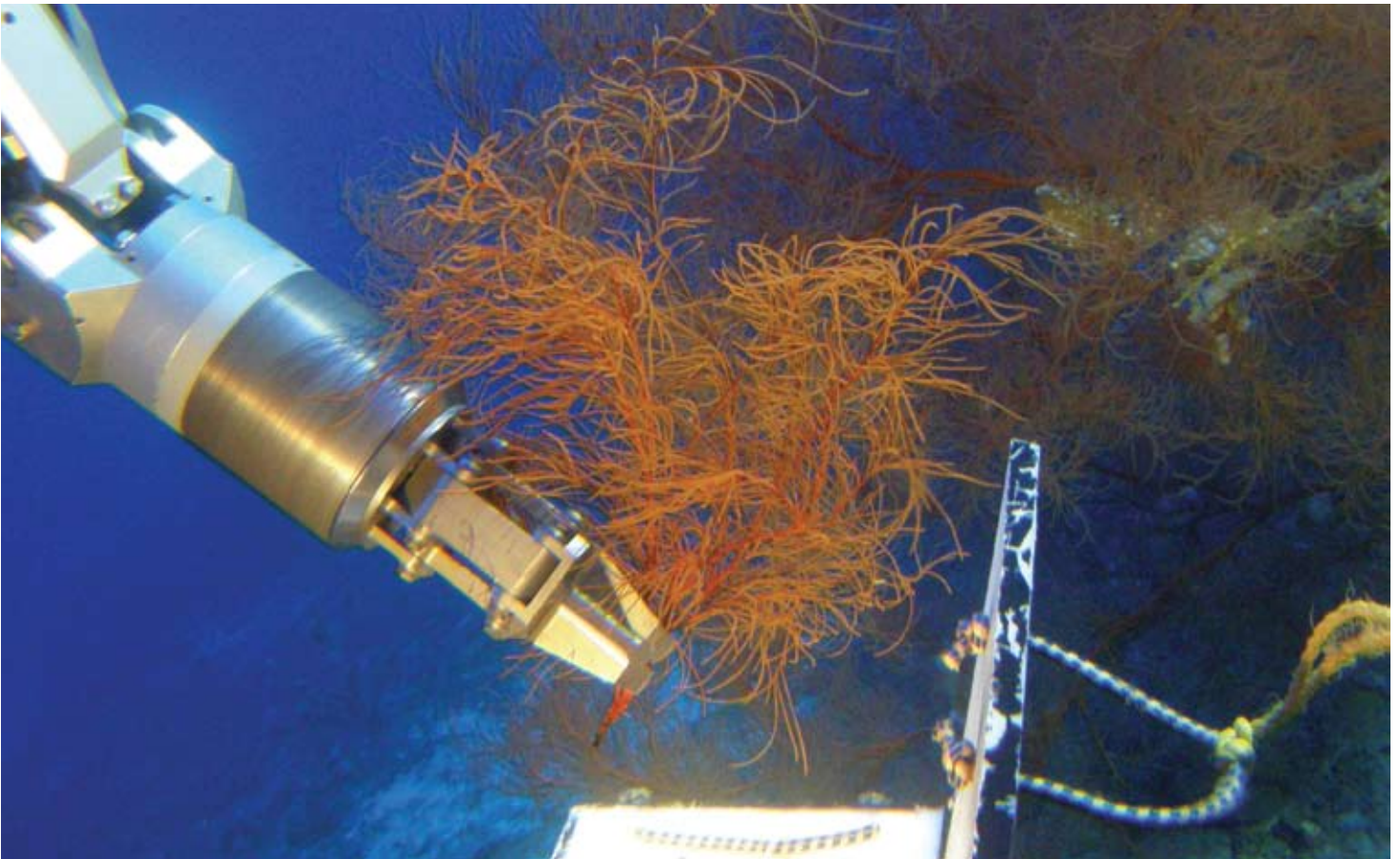
The Pisces IV , a 3-person, 2,000 m capable submersible, shown collecting a scientific sample of black coral, Anitpathes grandis .
