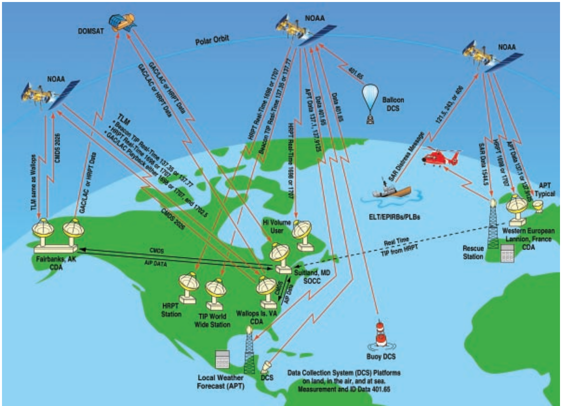
NOAA KLMNN' Spacecraft Communications Radio Frequency (RF) Links (frequencies are in MHz)
