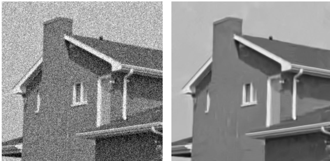
Fig. 5. Noisy ( \sigma = 25 ) grayscale House image and the BM3D estimate (PSNR 32.86 dB).
