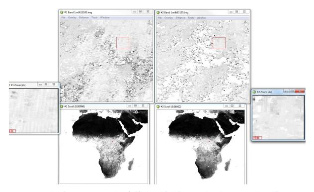
Figure 16: Examples of NDVI composite without (left) and with (right) view zenith angle constraint. Three different zoom-levels are shown for the same area. As can be seen in the image on the right, the angle constraint decreases the occurrence of artefacts, but increases the number of pixels without valid observation.
