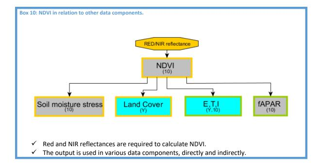
NDVI is based on the spectral reflectance of the red and near-infrared wavelengths of multispectral satellite data. It is calculated as follows:
