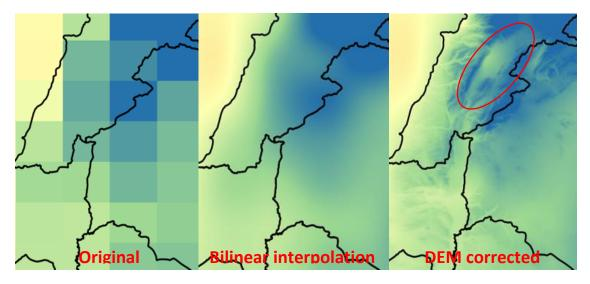
Figure 29: Example of coarse resolution global temperature data resampled for the Bekaa valley (circled) using a DEM. This example uses GEOS-5 temperature data.
