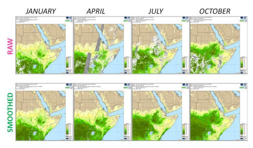
Figure 17: Example of original and smoothed NDVI for four dekads in 2010 from MODIS-250m over the Horn of Africa. Smoothing replaces all clouds and missing values with appropriate values.
