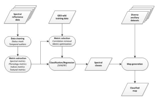
Figure 13: Schematic overview of the land cover classification processing chain. Different types of reference data as well as dekadal NDVI and multispectral remote sensing inputs are used to train a machine learning classifier. The input data vary across the different Levels.
