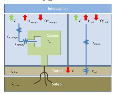
Figure 6: Schematic diagram illustrating the main concepts of the ETLook model, where two parallel Penman-Monteith equations are solved. For transpiration the coupling with the soil is made via the subsoil or root zone soil moisture content whereas for evaporation the coupling is made via the soil moisture content of the topsoil. Interception is the process where rainfall is intercepted by the leaves and evaporates directly from the leaves using energy that is not available for transpiration.
