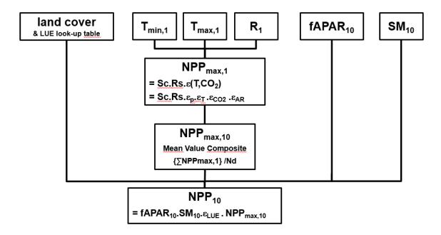
Figure 9: Detailed process flow of NPP. Daily NPP<sub>max</sub> is estimated based on meteorological data. At the end of each dekad, a mean value composite of these NPP<sub>max</sub> images is calculated. The final NPP<sub>10</sub> product is retrieved by the simple multiplication of the mean value composite NPP<sub>max</sub> with the fAPAR, soil moisture stress and the land cover dependent light use efficiency. (Eerens, 2004)
