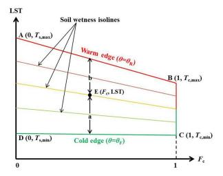
Figure 22: The trapezoidal vegetation coverage (F<sub>c</sub>) / land surface temperature (LST) space (transposed axis). Points A, B, C and D are estimated for each separate pixel using modified Penman-Monteith equations.
