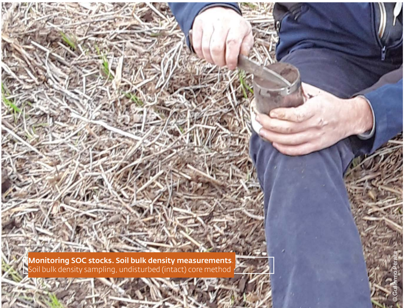
Monitoring SOC stocks. Soil bulk density measurements. Soil bulk density sampling, core method, using a rubber mallet
