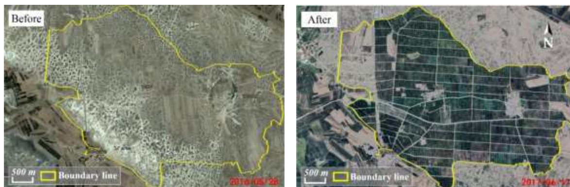
Figure 2. Landscape changes before and after amelioration with flue gas desulfurization gypsum shown in satellite remote sensing images.
