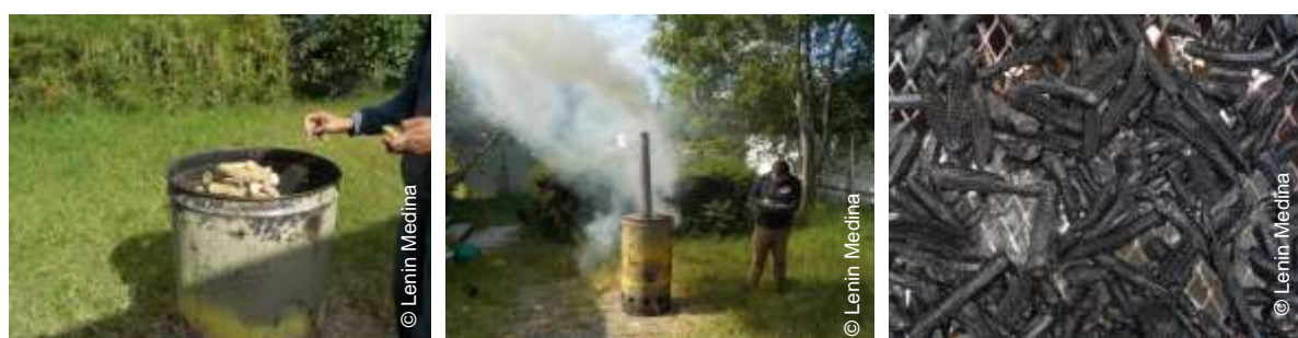
Figure 1. Manufacture of biochar from corn cobs using rustic equipment in the town of Tarimbaro Michoacan, Mexico
