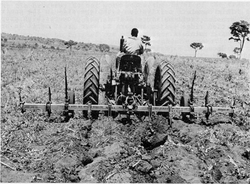
FIGURE 36. - Subsoiling previously ridged land, Uganda. (Photo Courtesy of National Institute of Agricultural Engineering U.K.)
