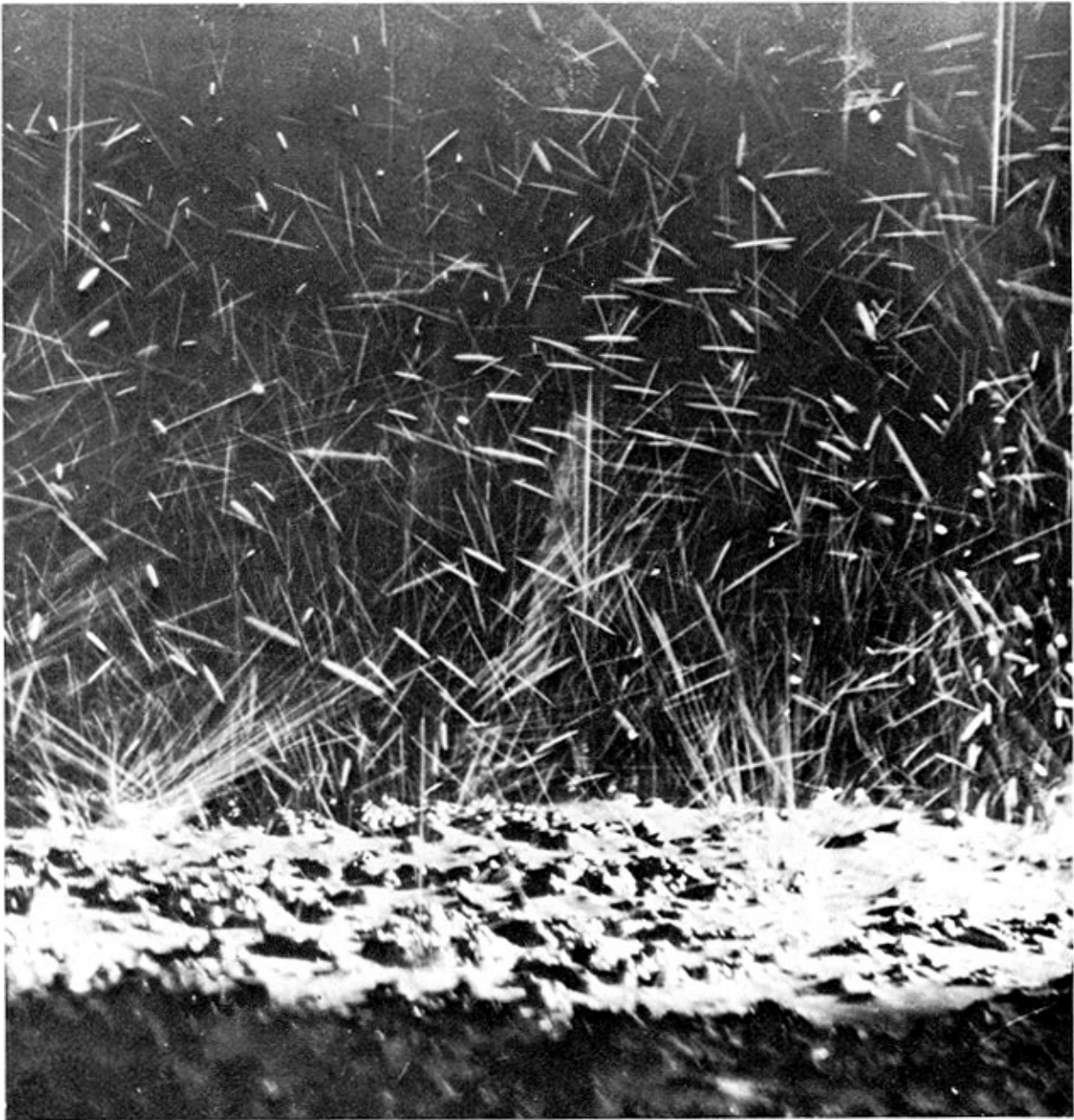
FIGURE 9. - Action of a multitude of raindrops on bare soil during a heavy rainstorm. (Photo USDA Soil Conservation Service (7).)
