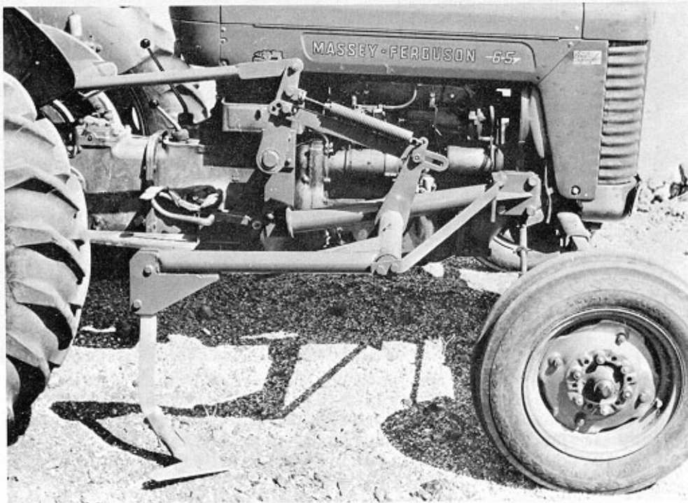
FIGURE 34- - Hydraulically lifted tie breaker. (Photo courtesy of Institute of Agricultural Engineering. U.K.)
