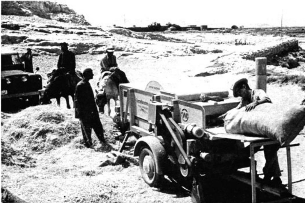
Picture 11. The experimental yields are threshed with a small machine not requiring cleaning after each sample. (Refer to Section 2.10.2)
