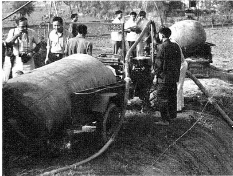
Plate 33. Biogas, stored in plastic bags is used to run irrigation pumps. (Mianyang, Sichuan Province).
