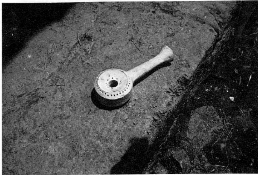
Plate 30. A locally made clay biogas burner (Anshi People's Commune, Zhejiang Province).
