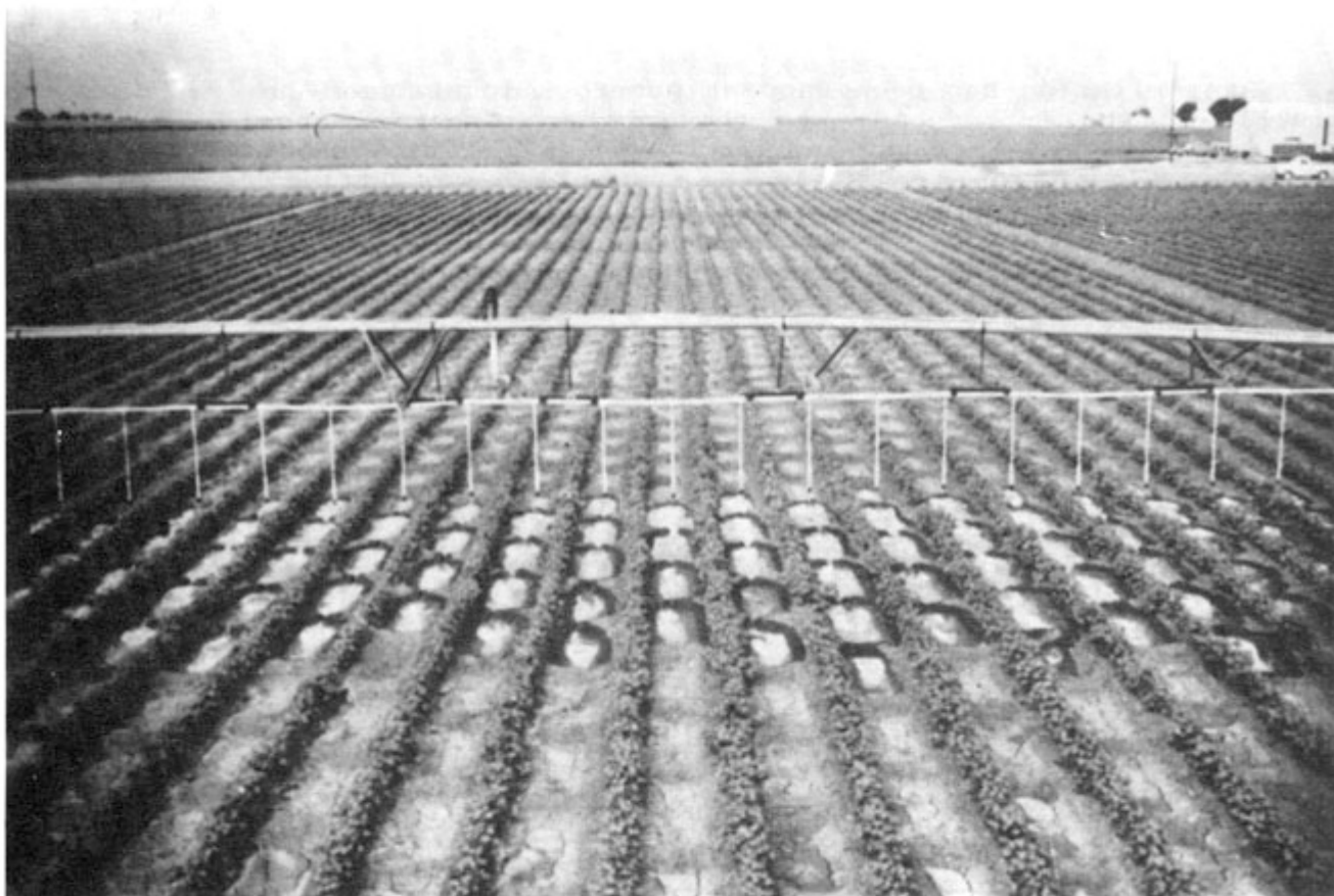
Fig. 94 Experimental low-pressure sprinkler irrigation system being used on basin-listed land (photo provided by W.M. Lyle, Texas Agric. Exp. Stn.)
