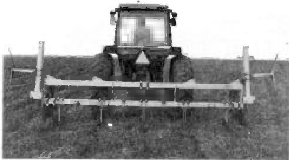
Fig. 75 Sweep implement: the sweeps (Fig. 76) undercut the surface to control weeds and retain most crop residues on the soil surface. The sweeps on each end could be turned down for use with a larger tractor
