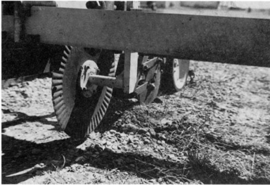
Fig. 90 Rippled coulter ahead of unit planter that can be used for no-tillage seeding of a crop
