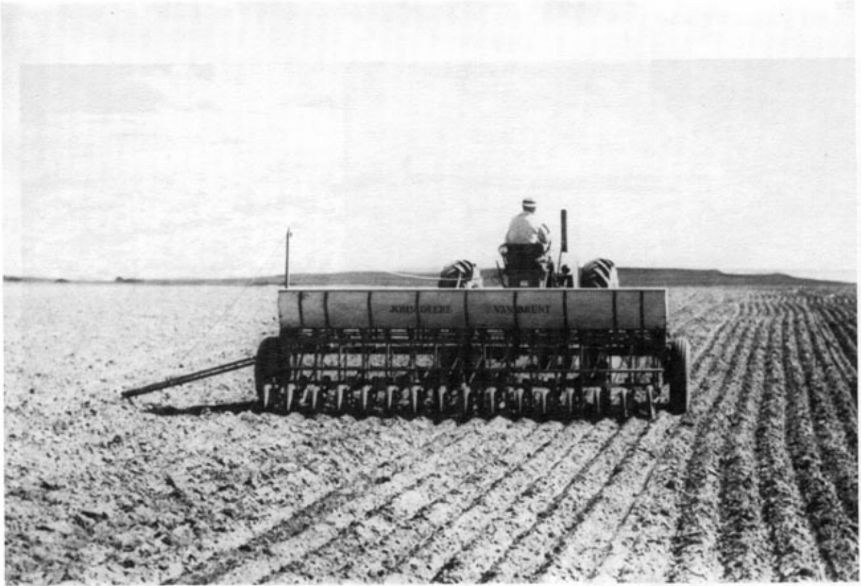
Fig. 119 Crop seeding with a semi-deep furrow drill. The ridges help control erosion (FAO photo)
