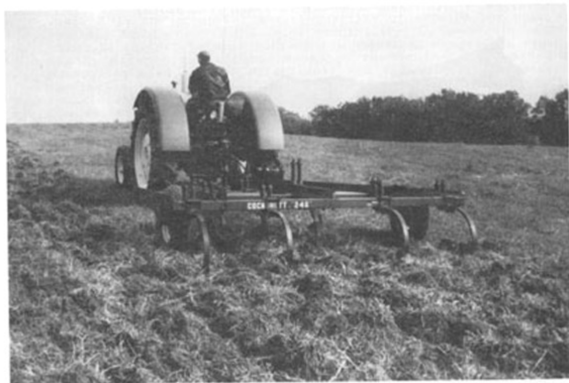
Fig. 17 A heavy-duty cultivator leaves a residue-covered, cloddy surface which reduces soil and water losses (FAO photo)
