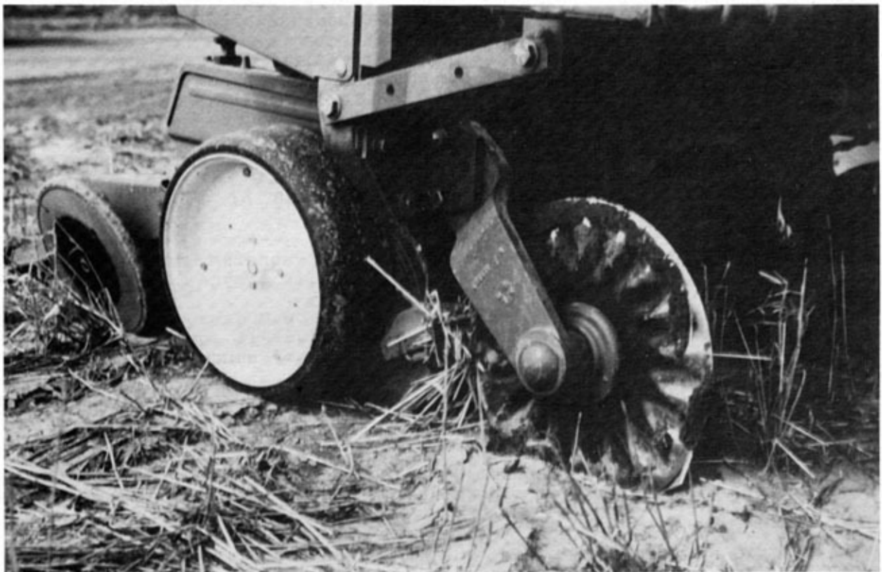
Fig. 133 Close-up view of unit planter for seeding row crops
