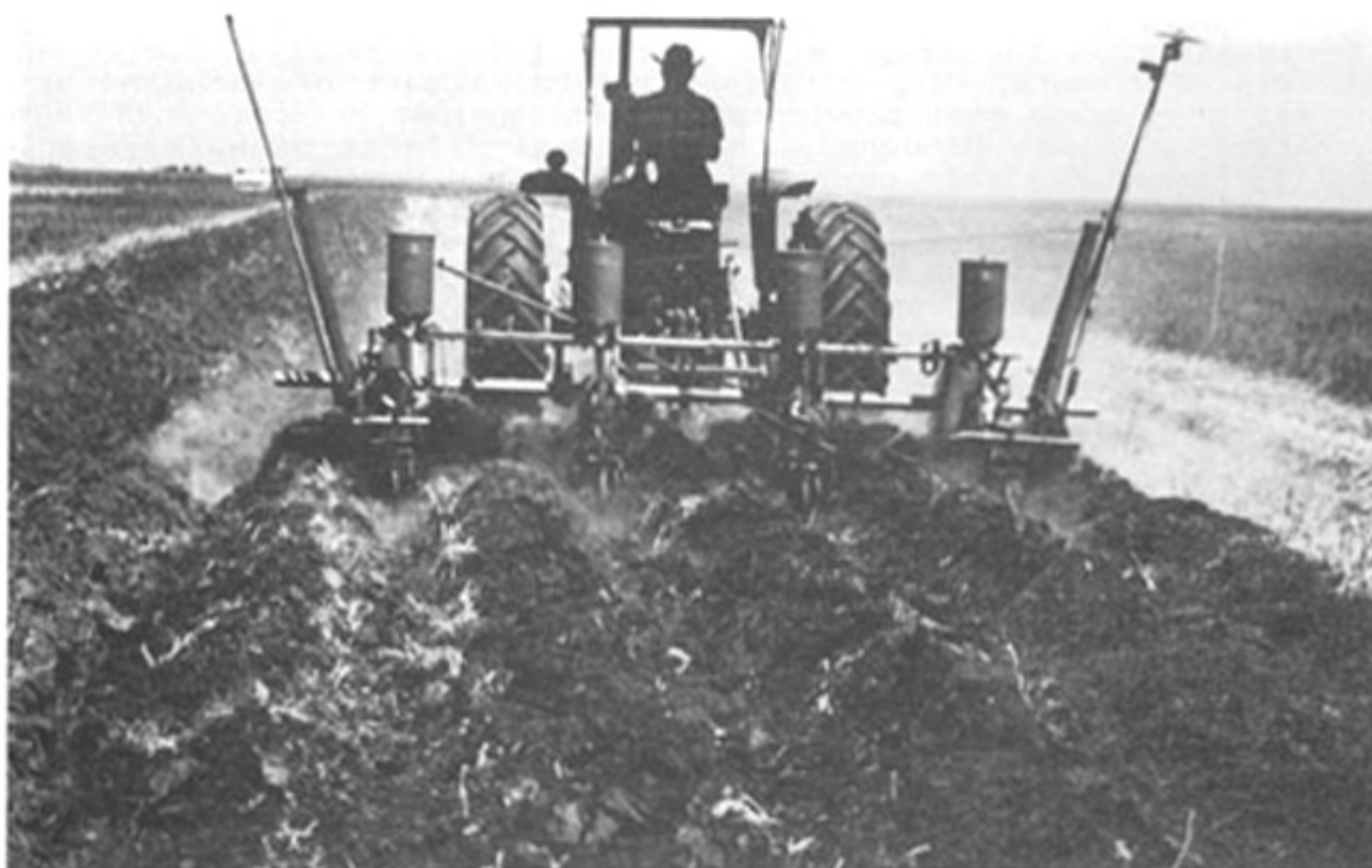
Fig. 36 Lister ploughing a field after wheat harvest. The attached planters could be used to seed a crop in conjunction with the tillage operation
