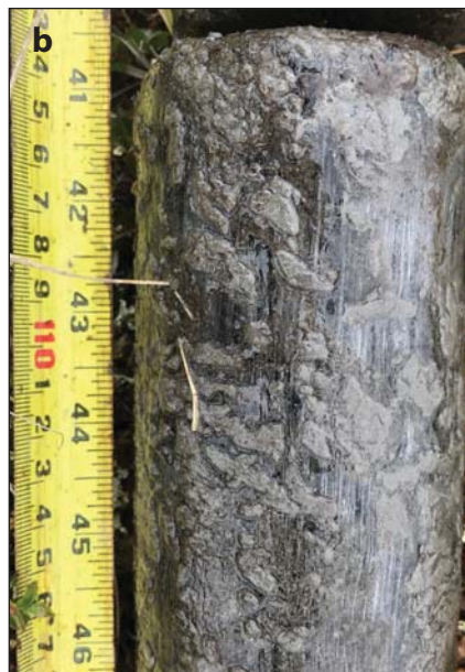
Figure A1.7. a. Borehole PLAY-10 was drilled with a SIPRE corer in a wet thaw lake basin with low-centered polygons, elevation 2.3 m a.s.l. b. Core shows ice-rich sandy silt with ataxitic cryostructure at depth of 104 to 117 cm. (Credit: M. Kanevskiy)
