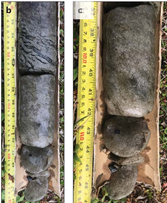
Figure A1.3 a. Borehole PLAY-1, elevation 3.1 m above sea level (a.s.l.), was drilled with the 3-inch diameter SIPRE corer in an ice-wedge trough. b-c. Photographs of the frozen core. At left ( b ), the protective intermediate layer of the upper permafrost (depth 76-93 cm) above the ice wedge is shown. Note inclined soil layers and ice lenses above the ice wedge ( b ) and gravel inclusions in wedge ice from ~105 cm ( c ). (Credit: M. Kanevskiy)
