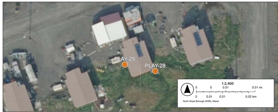
Figure A1.12. Two boreholes PLAY-28 and 29 were drilled with the Kovacs auger near the foundation of the TNHA house No. 810 on 28 June 2022, near the southeast and midwest piles respectively. (See Figure A1.1 for general location map.)
