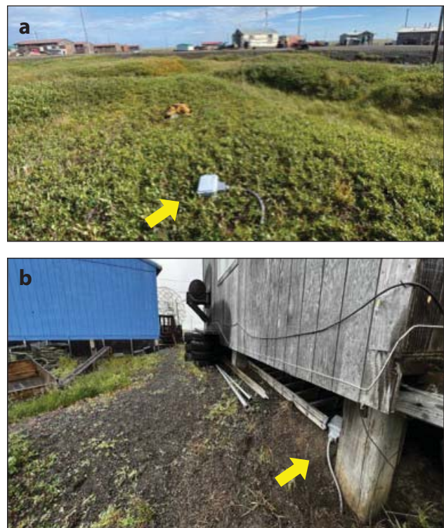
Figure 10. a. A ground temperature station installed on dry tundra in a natural site. b. A ground temperature station located on a foundation pile on a house without skirting. (Credits: D. Nicolisky)
