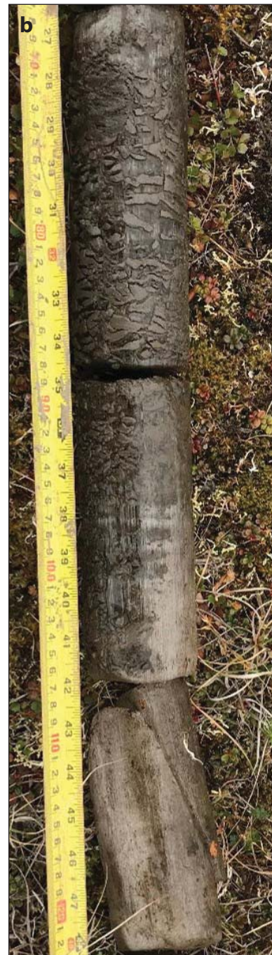
Figure A1.11. a. Borehole PLAY-26 at the center of a dry ice-wedge polygon, elevation 3.4 m a.s.l., was drilled with a SIPRE corer to 182 cm and with the Kovacs auger from 182 to 273 cm. b. The drilling analysis shows ice-rich silty sand from a depth of 68 cm and a buried ice wedge from 108 cm to 268 cm. (Credit: M. Kanevskiy)
