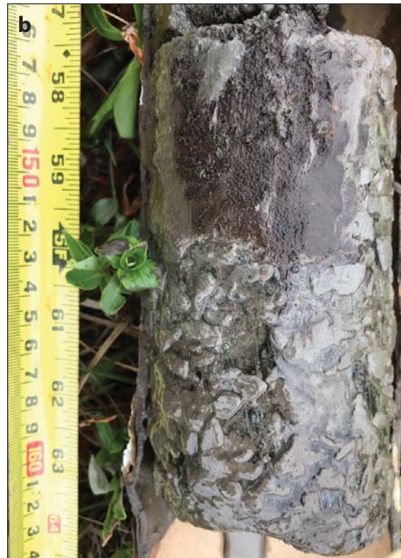
Figure A1.4 a. Borehole PLAY-3, elevation 9.2 m a.s.l., was drilled at the top of the baydzhherakh (thermokarst mound). b. Analysis of the core at a depth of 147-161 cm shows an ice-rich sandy silt with vertically oriented peat inclusions and ataxitic cryostructure in silt. (Credit: M. Kanevskiy)
