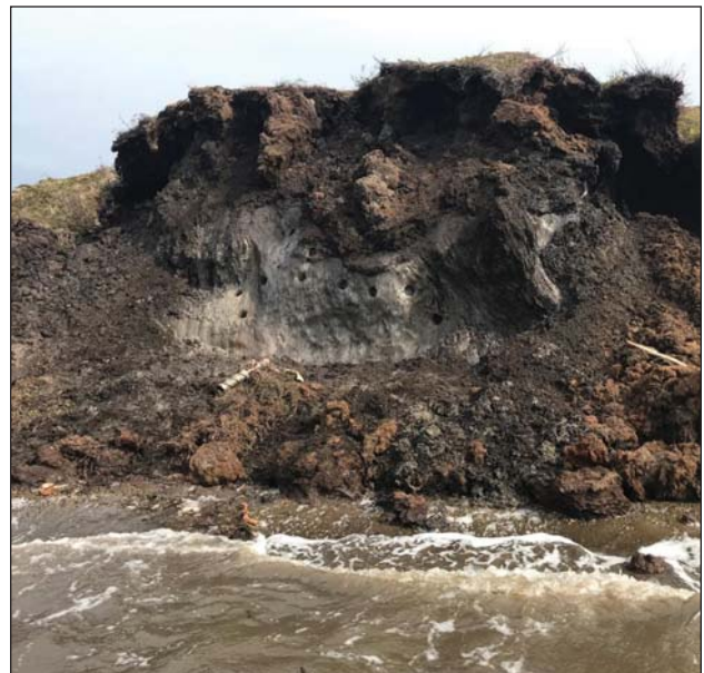
Figure A1.14. Sampling locations in the face of the coastal exposure PLAY-EXP to examine exposed wedge ice and adjacent frozen soils in the bluff behind the airport. The height of the bluff was measured at 4.8 m a.s.l. (which corresponds to the lower parts of yedoma slope), exposed part was ~0.6 to 2.8 m a.s.l. Exposed ice wedge ~2 m wide was enclosed in saline ice-rich very fine to fine silty sand with vertical peat inclusions. More likely, this ice wedge extends below sea level. (Credit: Mikhail Kanevskiy)
