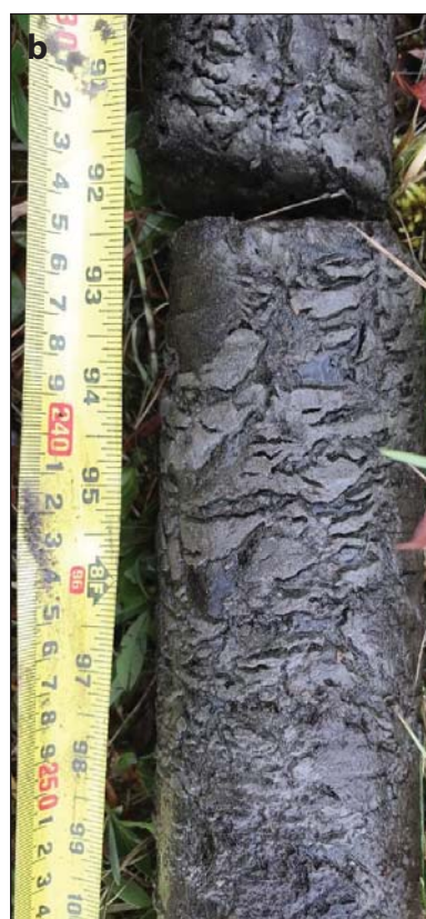
Figure A1.9. a. Borehole PLAY-12 at elevation 11.8 m a.s.l. was drilled with a SIPRE corer on a high surface north of the village. b. The core sample shows an ice-rich sandy silt with mainly ataxitic cryostructure at a depth of 230-255 cm. (Credit: M. Kanevskiy)
