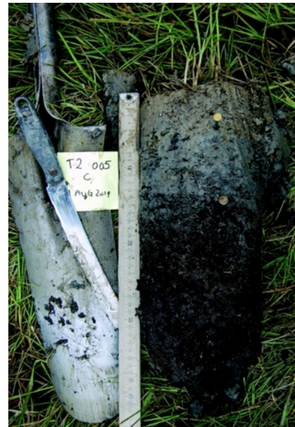
Figure 8. Soil plug taken from low-centered polygon in a roadside area. Note the 13-cm thick mineral surface horizon, which is the dust layer above the original organic surface horizon.
