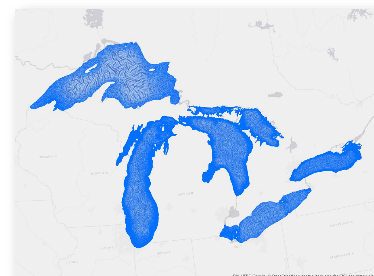
Figure 1. Next-Generation Great Lakes Operational Forecast System (GLOFS) on FVCOM grids
