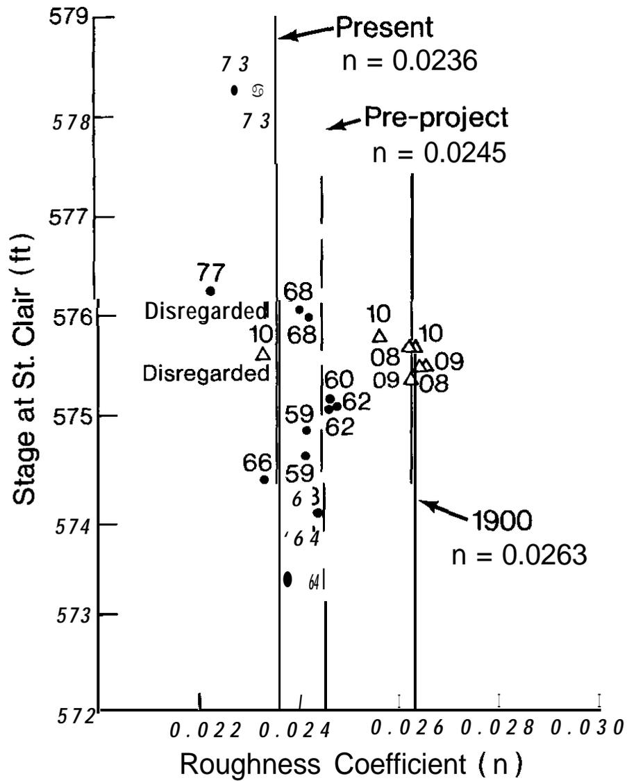
FIGURE 5.--Manning's roughness coefficients for MBR-SC reach.
