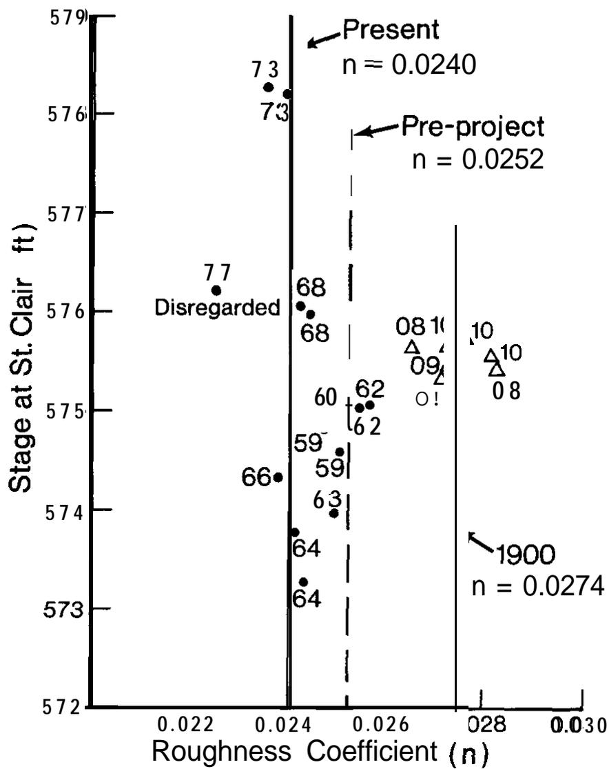
FIGURE 6.--Manning's roughness coefficients for *DD-SC reach*.
