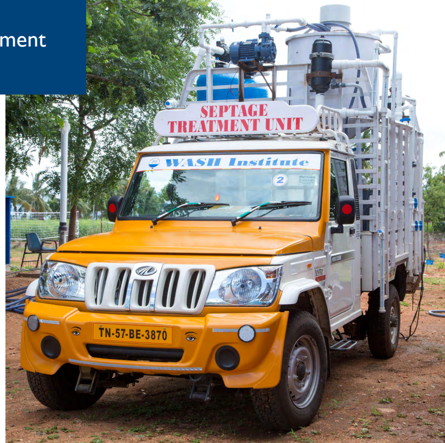
In India, a truck is outfitted with a Mobile Treatment Unit, a wastewater treatment system mounted on the bed of a truck that treats septic tanks onsite. Photo Credit: WASH Institute
