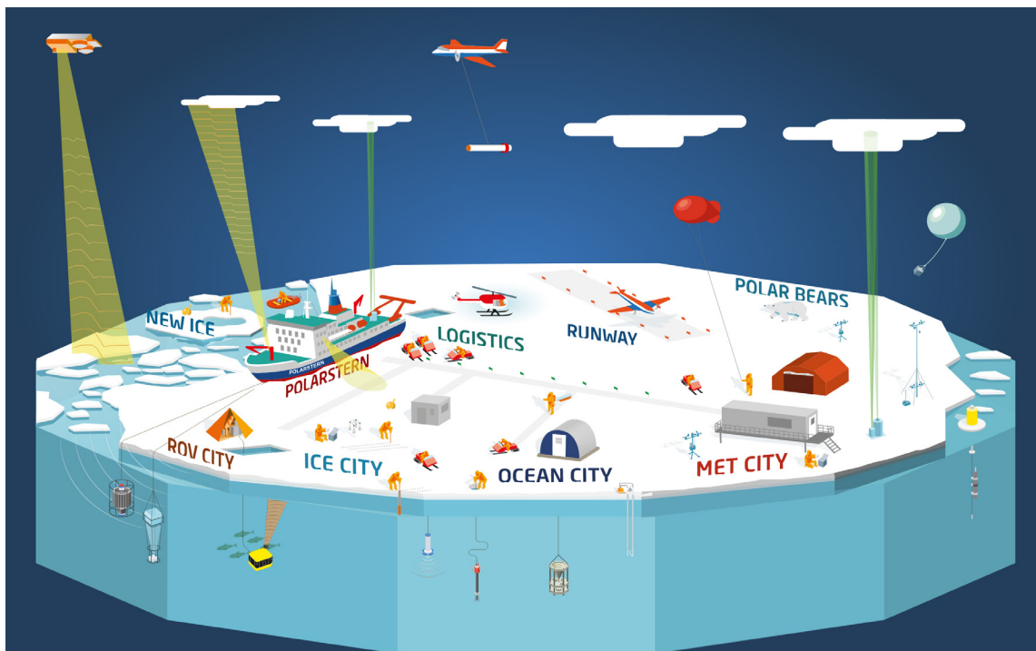
Illustration of the MOSAic expedition's Central Observatory, consisting of the main Ice Camp and R/V Polarstern anchored to the ice floe. Beyond surface and ice tethered installations, researchers used airborne, satellite, and under-ice instruments. Credit: Alfred Wegener Institute
