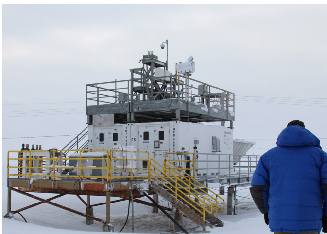
A visitor heads to ARM's radar wind profiler platform, which also hosts a sunphotometer, surface meteorology instrumentation and microwave radiometer profiler, at the ARM North Slope of Alaska (NSA) atmospheric observatory in Utqiagvik, Alaska. Credit: U.S. Department of Energy Atmospheric Radiation Measurement (ARM) user facility
