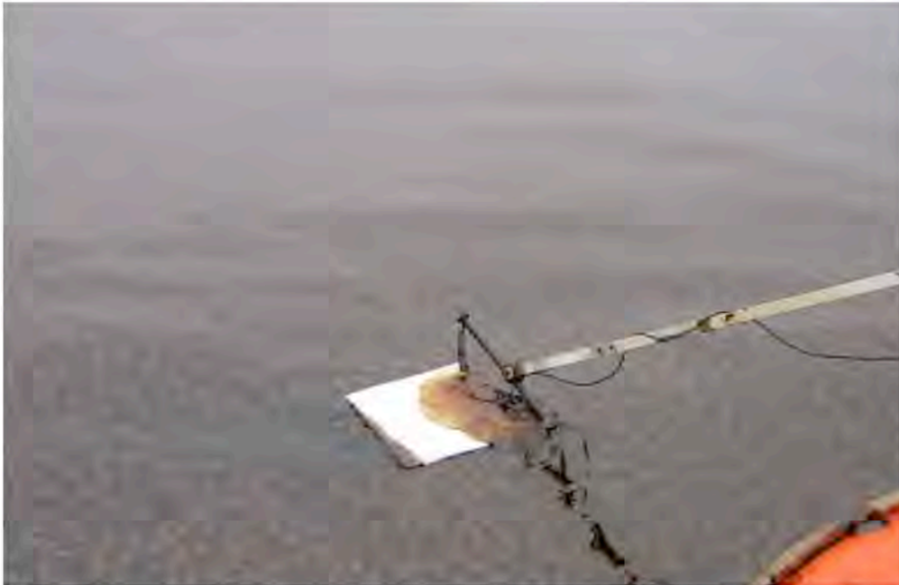
Figure 10. Discontinuous True Colour (Code 4, 50 to 200 \mu\text{m} ) as observed from a sampling boat
