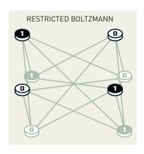
In a restricted Boltzmann machine, there are no connections between nodes in the same layer. The machines are frequently used in a chain, one after the other. After training the first restricted Boltzmann machine, the content of the hidden nodes is used to train the next machine, and so on.
