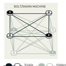
Geoffrey Hinton's Boltzmann machine is often constructed in two layers, where information is fed in and read out using a layer of *visible* nodes. They are connected to *hidden* nodes, which affect how the network functions in its entirety.
