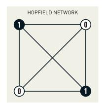
John Hopfield's associative memory is built so that all the nodes are connected to each other. Information is fed in and read out from all the nodes.
