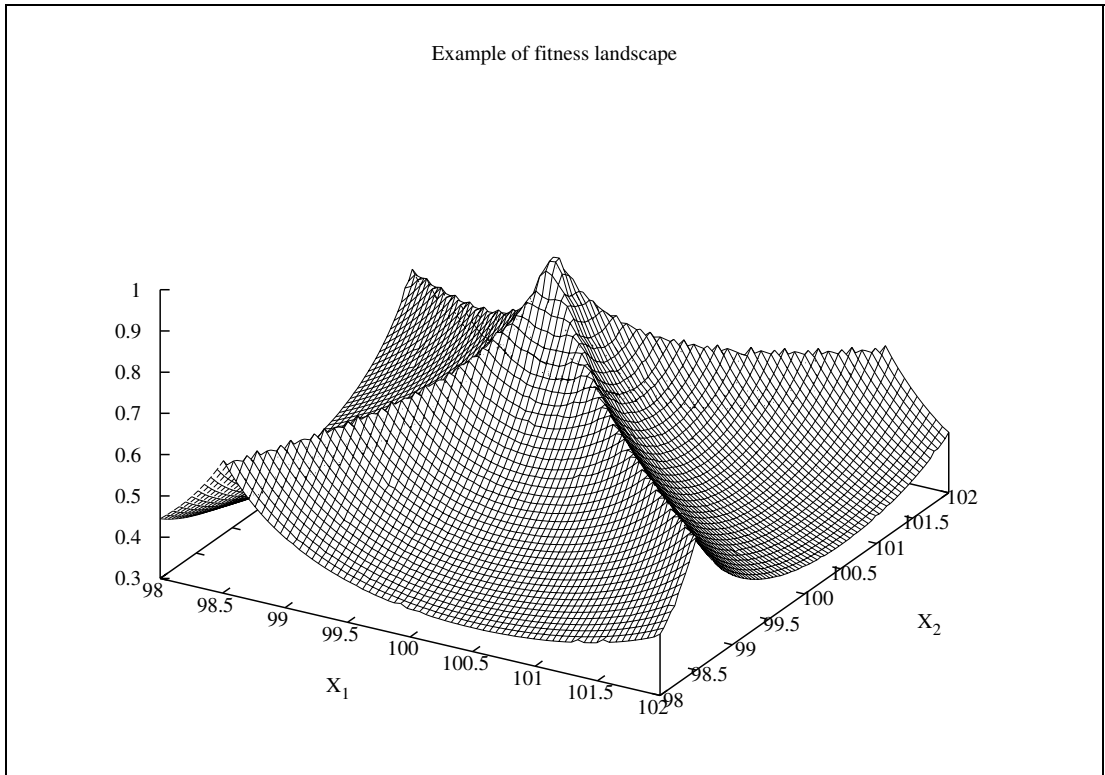
Figure 1: Fitness landscape for N = 2 with symmetric and relatively strong interdependency. Global optimum set at (100,100) with maximum fitness set to 1, and |a_{i,j}| = 0.7 . A hill-climbing strategy based on one-dimensional mutation corresponds to moves parallel to one of the axes. If, as in the figure, the ridges of the landscape are diagonal to the axes, they represent areas of local optima for one-dimensional search strategies. In fact, any vertical or diagonal step would force to “step down” from the ridge resulting in a fall of fitness. Only if the ridges are parallel to the axes ( a_{i,j} = 0 ) a one-dimensional search strategy can walk on the ridges and will always reach the global maximum.
